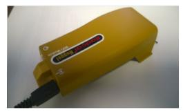
Press the power-on button of the Nugget. The Wi-Fi light will come on GRN then ORN. When it starts blinking orange quickly, the update is complete. Unplug the flash drive, press the Nugget power button to turn it off and then back on again. It is now ready to use.
