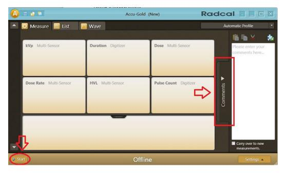
The *Comments* pane can be used to copy, cut and paste commands. Comments can be saved in the session along with any measurements and can optionally be carried over to the next measurement. The *Comments* pane can be accessed from all views. You can resize the pane by clicking and holding the *Comments* tab. A white line will appear on the tab. Drag the pane to the desired width and release.
