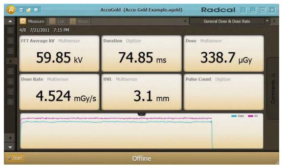
8. Make additional exposures as necessary. No data will be lost. You can review the previous measurements by clicking the **Up** and **Down** arrow buttons on the left side of the Measure screen.
