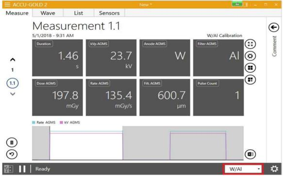
• You can now switch the anode filter to W/Rh and repeat the same exposure
