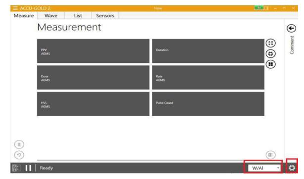
• Click on the Settings button on the bottom right and set "End of Exposure Delay" to 3 seconds. If additional time is required change to 5 seconds.
